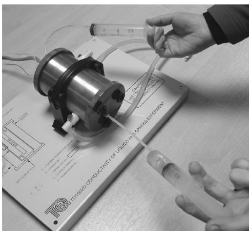
Figure 4. 7 Using the Syringes to add Fluid
