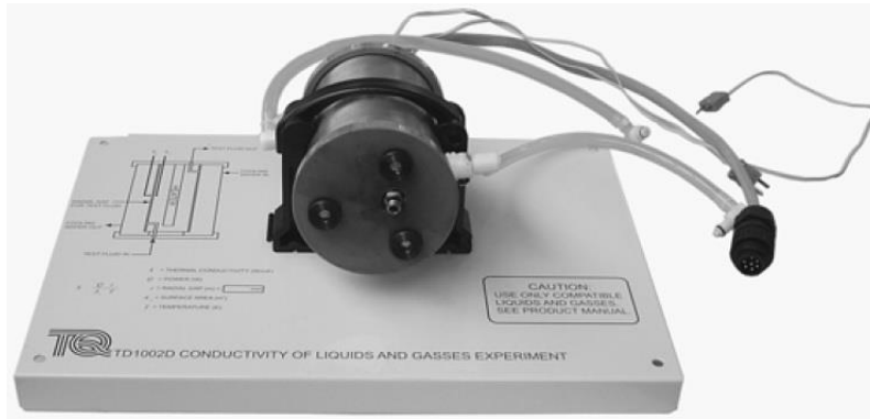
Figure 4. 2 The Conductivity of Liquids and Gasses Experiment
